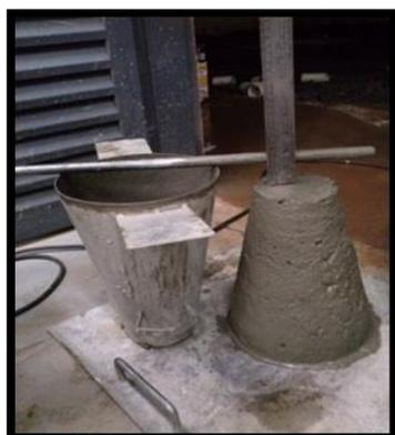
Figura 1: Slump Test
